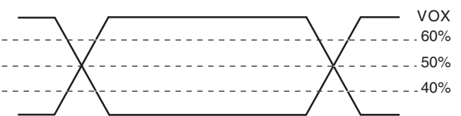
OUTPUT CROSSOVER VOLTAGE
